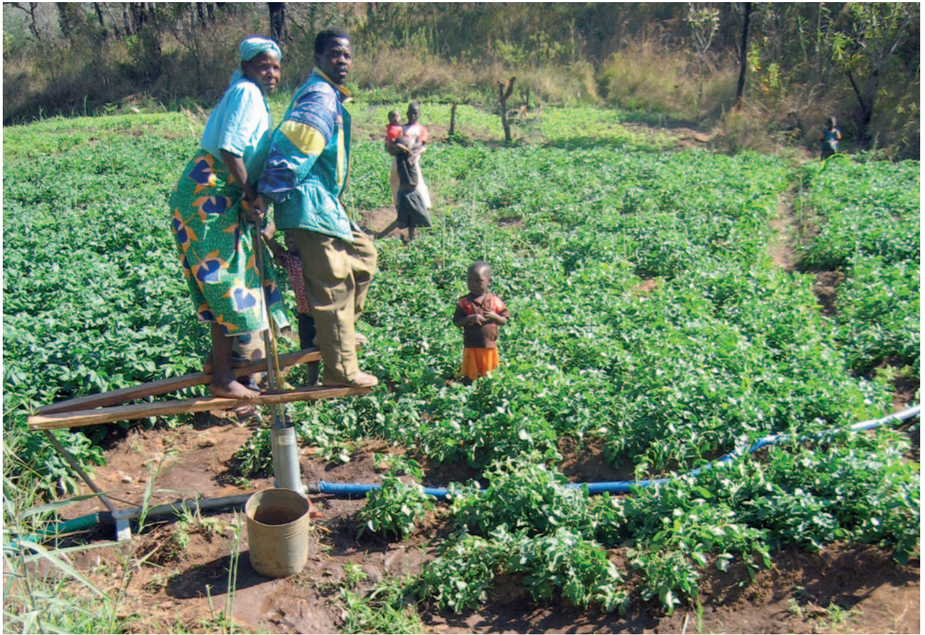
The village of Chiandane uses a treadle pump next to a small stream to irrigate their crops. Photo: Lorne Kletke
